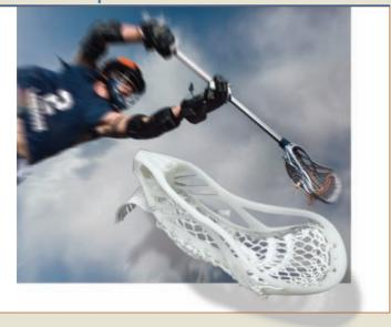
During testing, a lacrosse stick head prototype (Figure 4) was truly put through its paces, from wind tunnel testing to live-action performance trials with lacrosse players shooting balls at speeds of up to 90 mph at the prototype part
